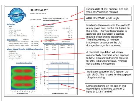
The radiant energy, or dosage, delivered to a coil surface is dependent on UV intensity, the duration of exposure, and the lamp to coil distance.
